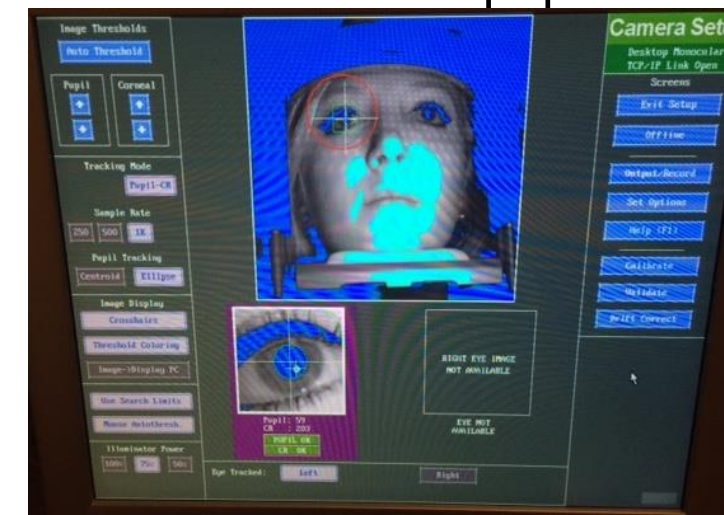
Figure 2. The examiner's view of the participant's pupil from the EyeLink's infrared camera.
