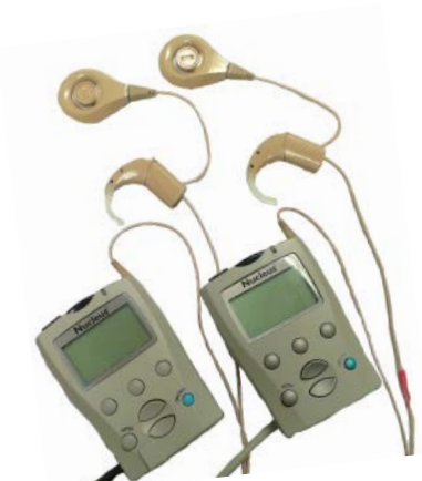
Figure 1: L34 Speech Processors which allow for the synchronization of timing between implants.
