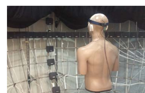
Fig. 1. An array of 37 loudspeakers separated by 5^\circ in azimuth ( -90^\circ to +90^\circ ).
