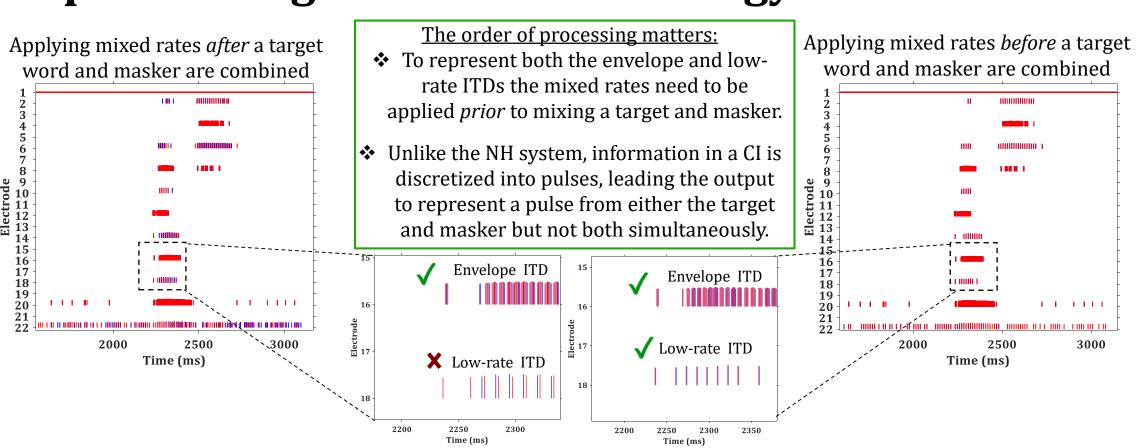
**Figure 8:** Electrodogram of the word "GOOSE" in +12 dB SNR SSN with a 1000 μs ITD. Stimulus was processed using two different methods in a CIS-like strategy.
