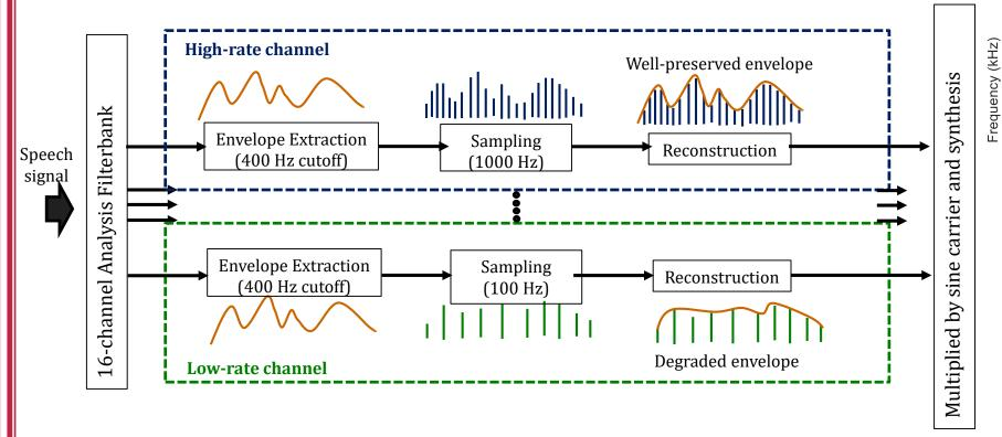
Figure 3: Schematic for vocoding mixed rates. Low-rate channels were implemented by reducing the sampling rate to 100 Hz. High-rate channels were sampled at 1000 Hz. Figure redrawn from [5].
