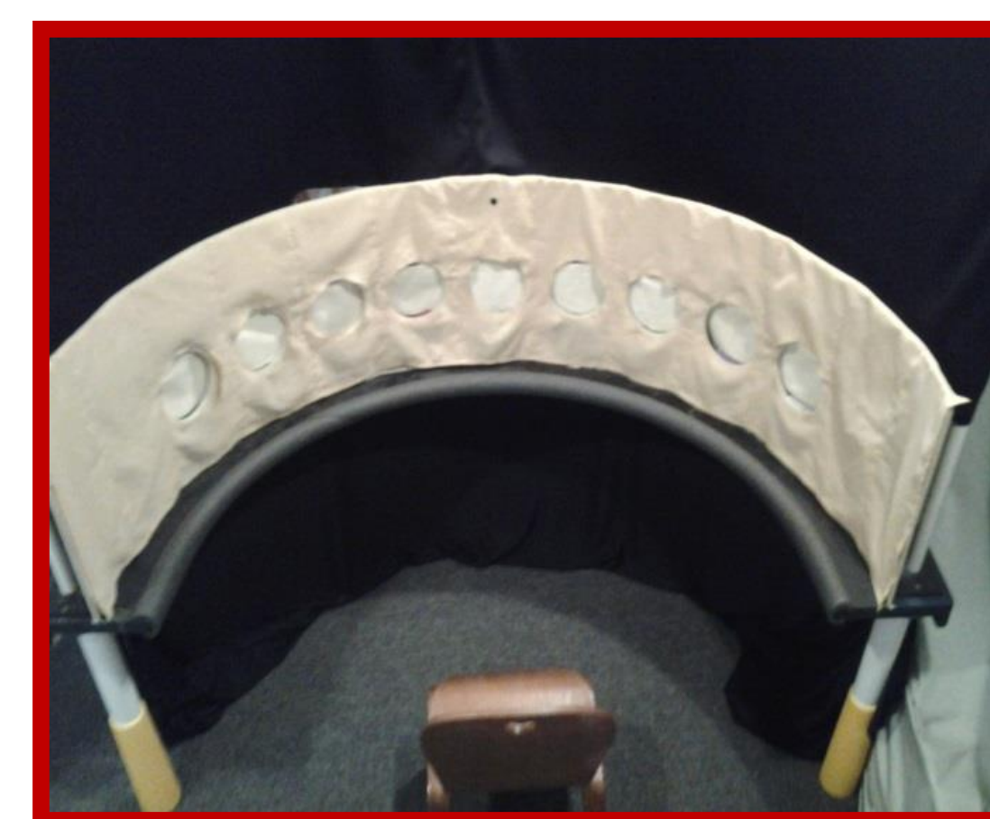
Figure 2: Testing apparatus was an arc spanning -60° to +60° azimuth. There was a loudspeaker behind each hole.
